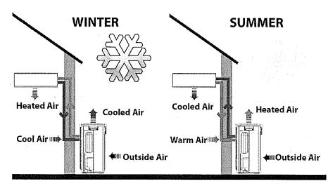
Heat pumps do not generate heat but extract it from one body of air and transfer it to another. They use the same principle as your fridge, compressing gas and then allowing it to expand, extracting heat as it does so.
